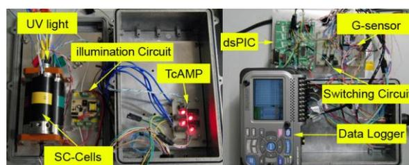
**Fig. 3** Components of the photoreactor
