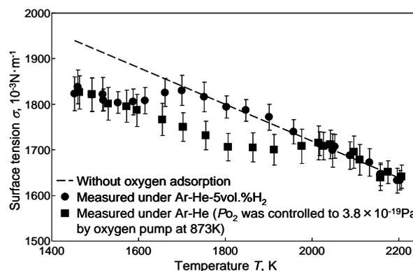
**Fig. 1** Surface tension of molten nickel measured under Ar-He gas processed by oxygen pump and under Ar-He-5vol.%H<sub>2</sub> gas. The surface tension of pure state is expected from the plots as a dashed line
