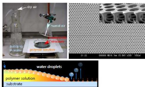
**Fig. 1** Fabrication of a honey comb film
