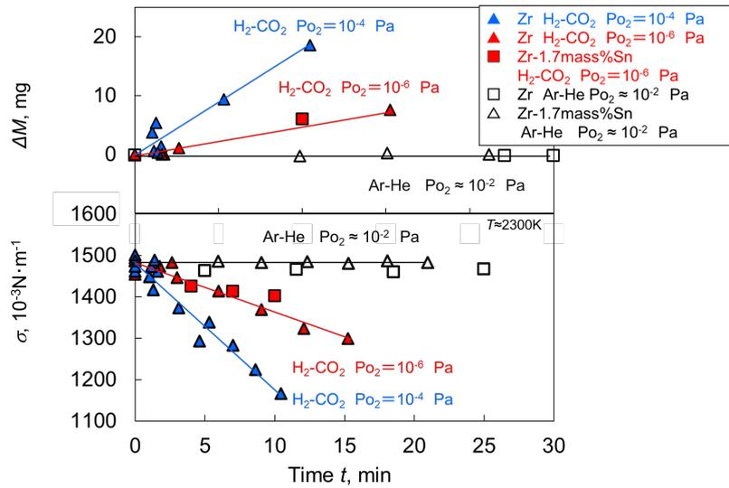
**Figure 1.** Variations of sample mass and corresponding the surface tension of molten zirconium (△, ▲, ▲) and Zr-1.7mass%Sn (□, ■, ■) with time when the sample was maintained at 2300 K under atmospheric gases of Ar-He and Ar-He-H<sub>2</sub>-CO<sub>2</sub>.
