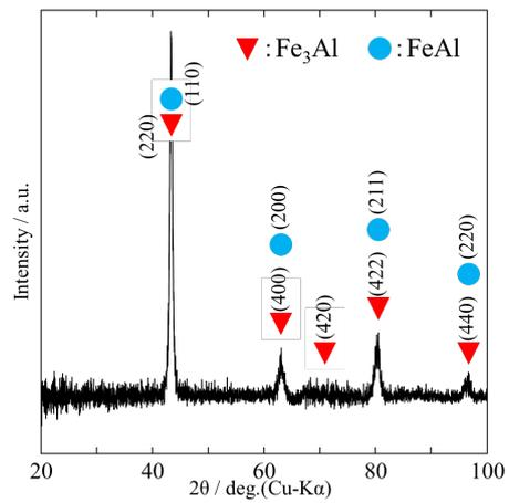
**Figure 2.** XRD analysis result of Fe-Al sample.
