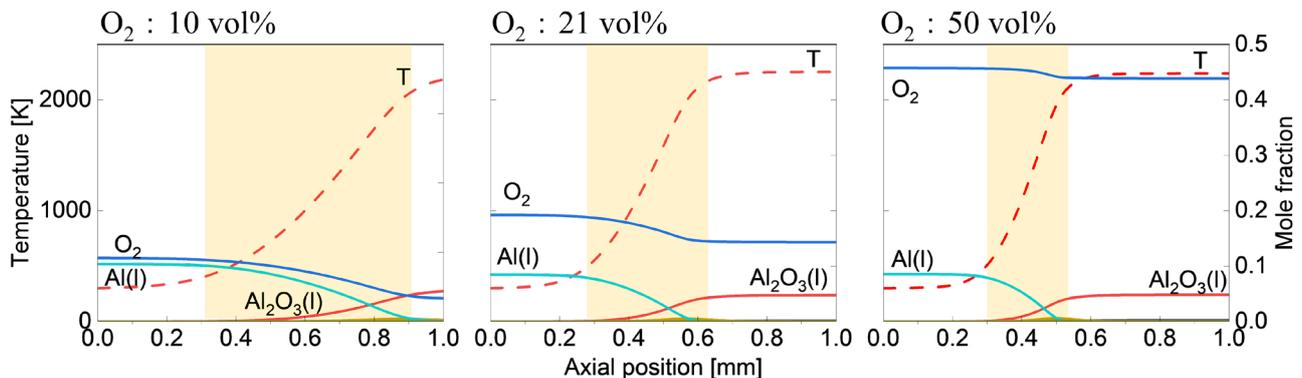
Figure 2. Aluminum flame structures (O<sub>2</sub> : 10, 21, 50 vol%)
