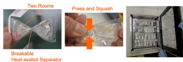
Figure 2 Sample bag used in the space experiment; two bags (3 mL) are connected by a bulkhead, and the two liquids are mixed by crushing the whole bag. The sample is set in a device equipped with a UV-LED and gelatinized by UV irradiation.
