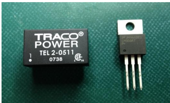
Fig. 5 DC-DC converter (left) and series regulator (right)
