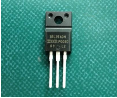
Fig. 4 FET (IRLI540NPbF (International Rectifier), TO-220 Full-Pak Package)
