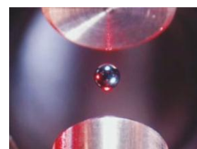
Fig. 4 Electrostatic Levitation of EM( \phi 2mm glassy carbon)
