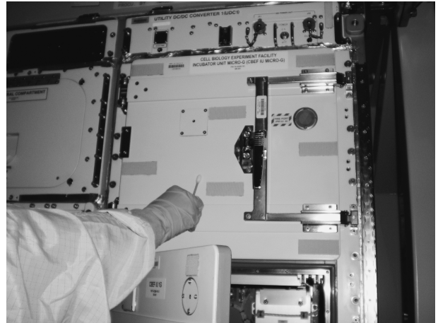
Fig. 3 Zero-time reference samples have been collected from the surface and inside of the SAIBO rack in SSPF, Kennedy Space Center at 11 th June, 2007.
