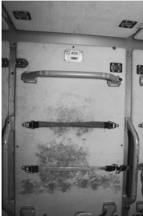
Fig. 1 An example of microbial contamination on one of the interior panels on board ISS. (NASA Image: ISS010E11563, © NASA)
