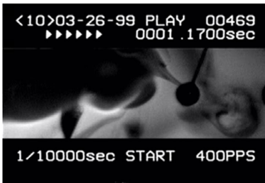
Fig. 5 (Movie) Generation of fuel vapor jet at 3.0 MPa for n-decane 11) . Droplet diameter is 1mm.
