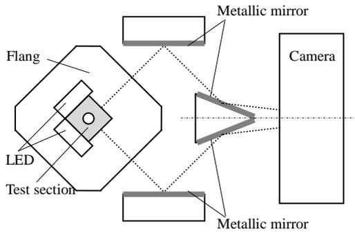
**Fig. 2** Arrangement of the optical system.
