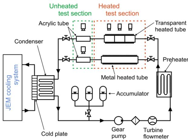
Fig. 5 Outline of test loop for ISS flow boiling experiment "TPF".
