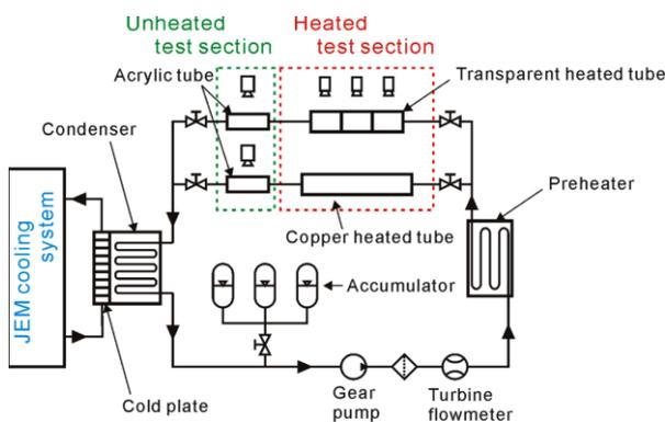
Fig. 1 Outline of test loop for ISS flow boiling experiment.
