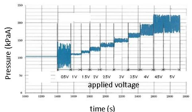
Fig. 2 Pressure fluctuation with applied voltage to the pump
