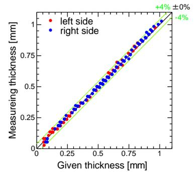
**Fig. 6** Comparison of liquid thickness between measured result from image and given values using calibration rod.
