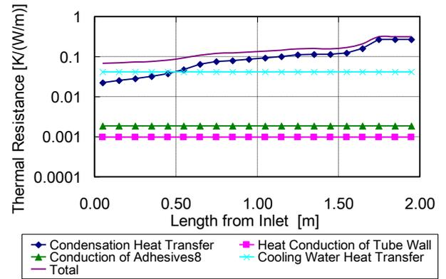
**Fig.3** Thermal resistance at local point
