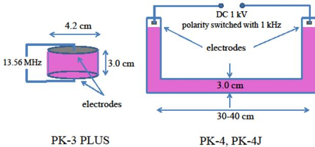
**Fig.1** In PK-3 PLUS (left), plasma is generated by rf discharge. In PK-4 and PK-4J (right), dc discharge with polarity switching generates plasma and behavior of dust particles is observed in the central straight part which is a long cylinder.
