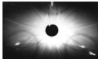
Fig. 2 Kikuchi Kossel Diffraction
