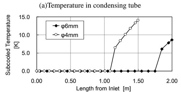
**Fig.4** Temperature and sub-cool temperature resistance at local point
