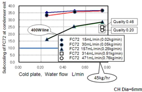
**Fig.6** Liquid subcooling of FC72 at exit of condenser tube
