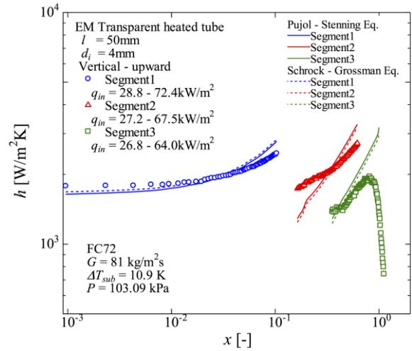
**Fig. 4** the relation between exit quality and heat transfer coefficients at each segment during flow boiling experiment by using transparent heated test section in EM facility.
