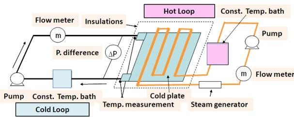
**Fig.5** Ground test loop of condenser system
