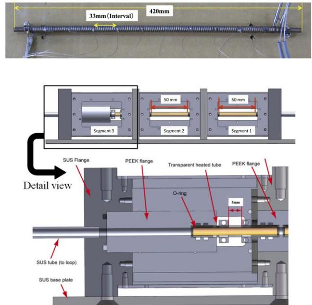
Fig. 2 Images of the metal heated tube section (Top) and the transparent heated section (Bottom).
