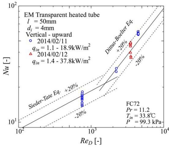
**Fig. 3** Single-phase heat transfer at Segment 1 in the transparent heated tube section.
