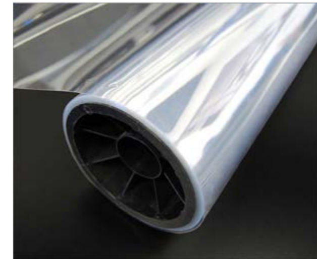
Airtight seal: 0.1 mm thick mylar (plastic sheet)
