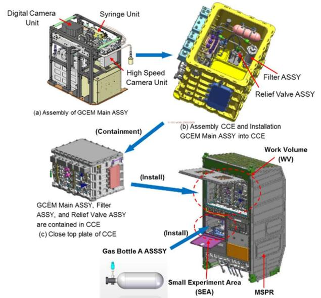
**Fig. 3** Installation procedure of the GCEM into the MSPR.
