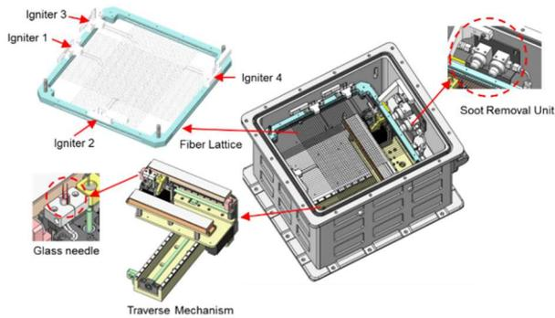
**Fig. 2** Schematic of the components inside the Small Combustion Vessel.
