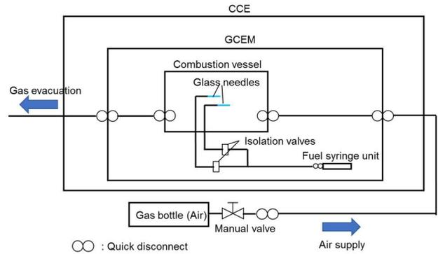
Fig. 18 Schematic on the fluid system lines (simplified) of GCEM and CCE.
