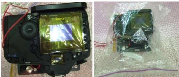
**Fig. 5** Launch configuration of the Digital Camera Unit ((C) JAXA).
