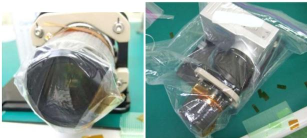
**Fig. 4** Launch configuration of the High-Speed Camera Unit ((C) JAXA).
