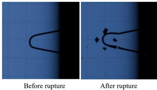
Fig. 22 Photo of the igniter-2 ((C) JAXA/Yamaguchi Univ.).
