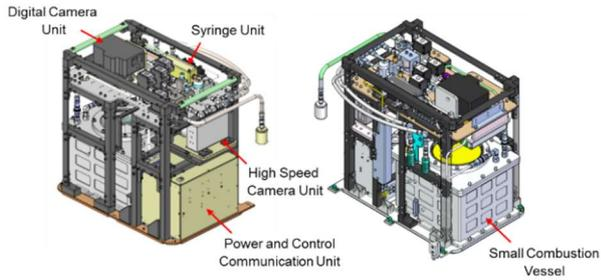
**Fig. 1** Schematic of the GCEM.
