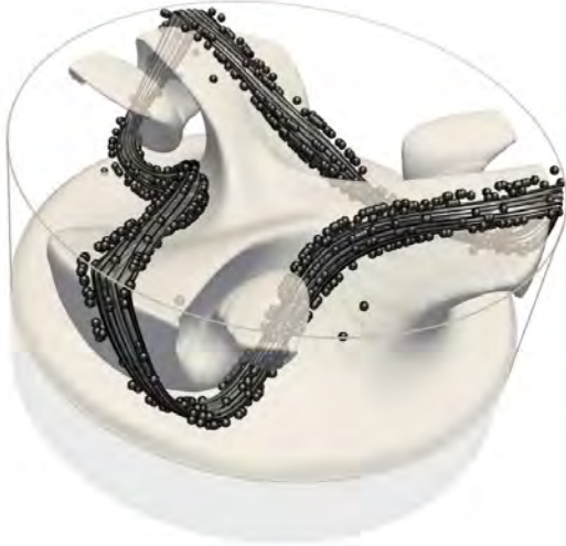
Fig. 6 A finite-size Lagrangian coherent structure (PAS) made by 1000 particles (dark spheres) forms in a thin KAM torus (not shown) slightly outside of the main KAM torus (dark-gray) for \Delta = 0.00552 , \Gamma = 0.68 , Re = 1600 and Pr = 28 . The temperature iso-surface \theta = 1/2 (light-gray) of the hydrothermal wave is strongly affected by the flow. The structure is shown at t = 3d^2/\kappa after particle initialization at random positions. The figure is taken from Romanò and Kuhlmann. 26)
