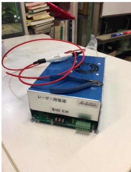
Fig. 2 Power supply for the CO<sub>2</sub> Laser.
