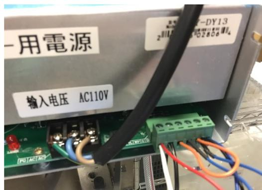
Fig. 5 Input terminal of power supply. Left (black): AC110V, Right (green): control signal.
