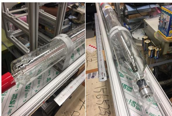
Fig. 3 Optical window and mirror of CO<sub>2</sub> Laser.
