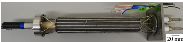
Fig. 1 Photograph of the shear cell same as used in the Foton mission.
