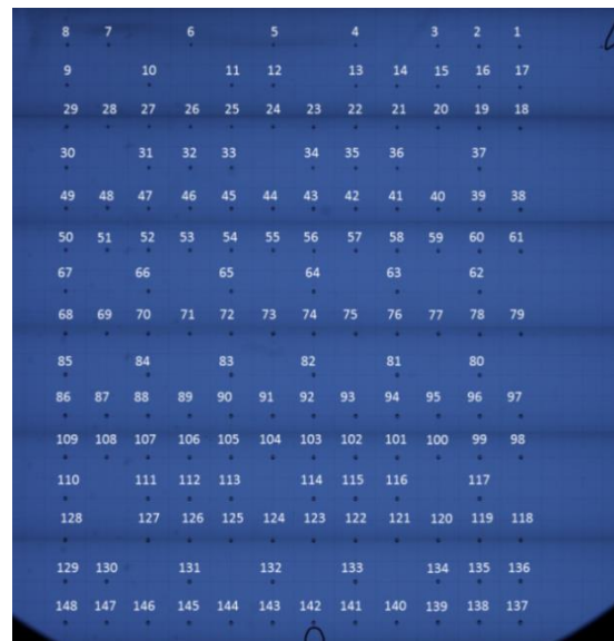
Fig. 3 Droplet arrangement on SiC-fiber lattice and droplet identification numbers.
