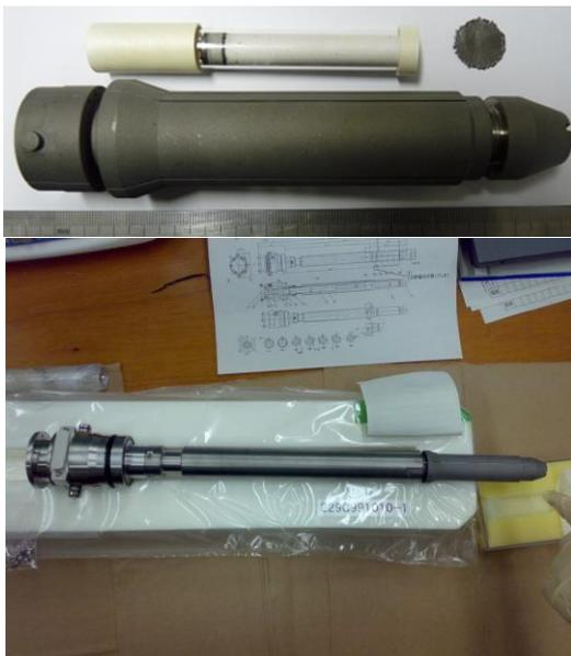
Fig. 5 Prototype of sample cartridge: (above) sample part and ampoule, (below) whole image.
