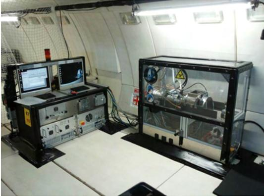
**Fig. 1** Photograph of the X-RISE facility aboard the A300 Zero-G of NOVESPACE. The rack on the left hand side hosts the experiment control equipment, whereas in the rack on the right hand side, the X-ray experiment unit is located.
