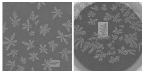
**Fig. 7** Radiographs recorded with the X-RISE facility under terrestrial conditions during the solidification of an Al-Ge alloy. The image on the left was taken under vertical configuration (quasi 2D sample perpendicular to the gravitational force). The image on the right was taken in horizontal alignment of X-RISE. Here the gravity vector point from top to the bottom of the image. The diameter of the circular samples is 12 mm.
