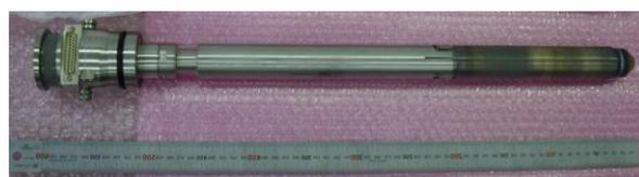
**Fig. 4** Outer view of a space-processed cartridge. The brown part is a heated part.
