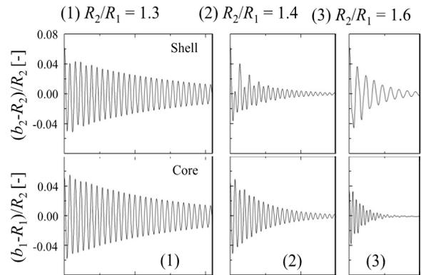
**Fig. 1** Effects of radius ratio of shell to core liquids on oscillation behaviors of compound droplets for the case of viscosity ratio of 3.9<sup>7</sup>).
