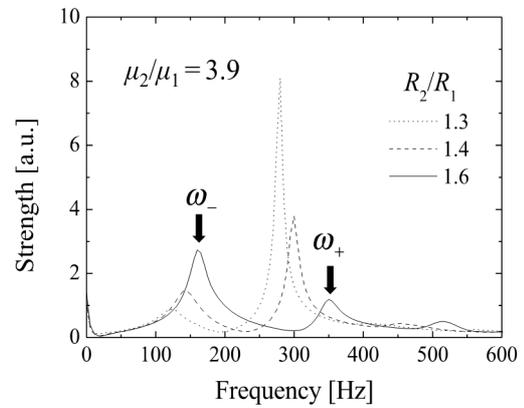
**Fig. 2** Effect of radius ratio of shell to core liquids on frequency spectrum of a compound droplet for the case of viscosity ratios of 3.9<sup>7</sup>).
