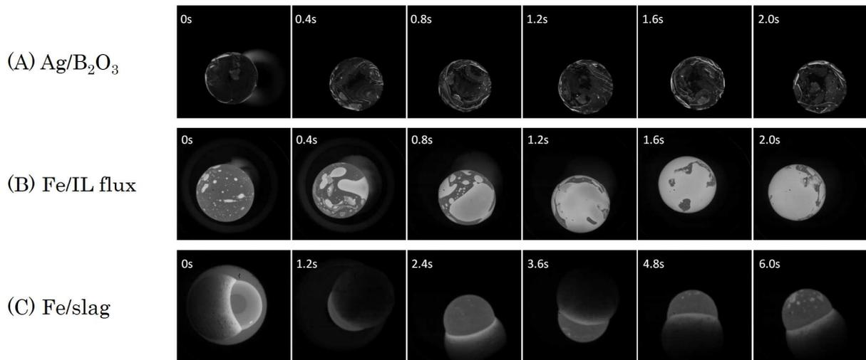
**Fig. 3** Top views of electromagnetically levitated metal/oxide sample under  $\mu$ G condition. (A) Ag/B<sub>2</sub>O<sub>3</sub>, (B)Fe/Ilmenite type welding flux, (C)Fe/Smelting slag (SiO<sub>2</sub>-CaO-Al<sub>2</sub>O<sub>3</sub> base)<sup>8</sup>).
