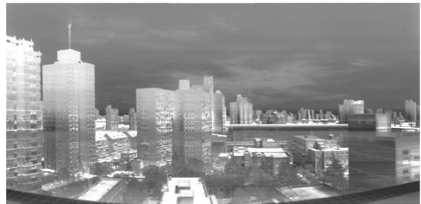
Fig. 5 Outdoor image in TIR band of spectral imager.
