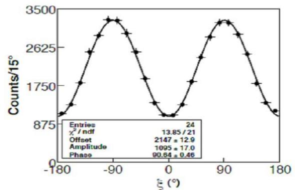
**Fig. 2** Modulation curve measured with 100 % polarized hard X-ray beam at 200 KeV.
