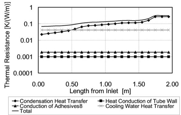
**Fig.4** Thermal resistance at local point
