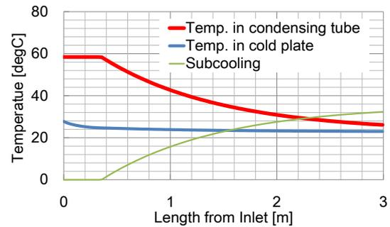
**Fig.10** An example for calculated result of temperature distribution in condenser and cold plate on flight test condition
