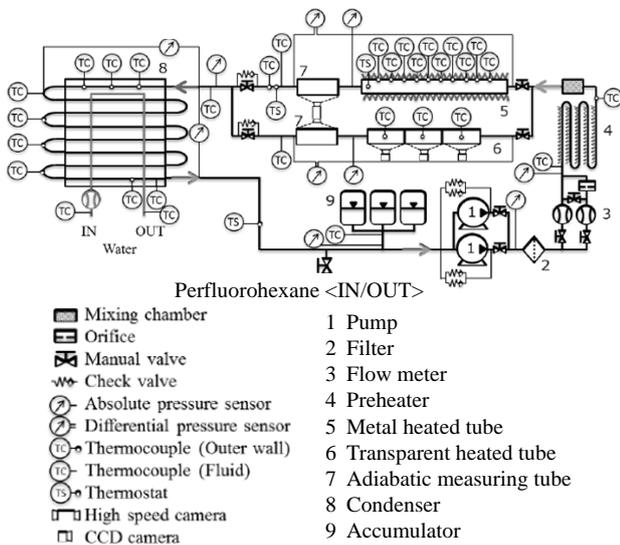
Fig.1 Schematic Diagram of TPF Experimental Loop<sup>5)</sup>
