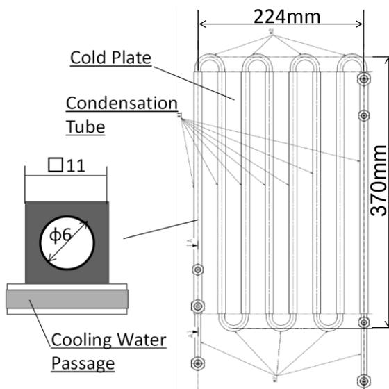
Fig.2 Structure of Condenser for TPF Experimental Fluid Loop
