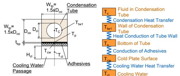
Fig. 3 Arithmetic Thermal Model of Condenser
