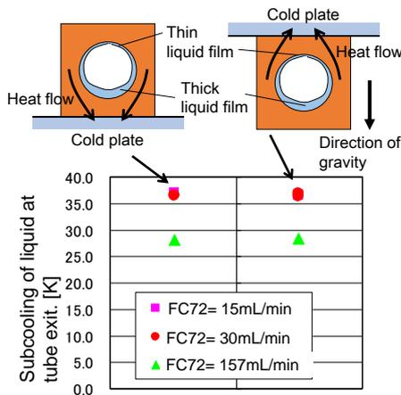
Fig.8 Effect of Orientation of Condenser on Thermal Performance
