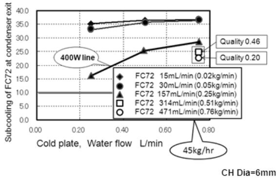
Fig.7 Liquid Subcooling of FC72 at Exit of Condenser Tube
