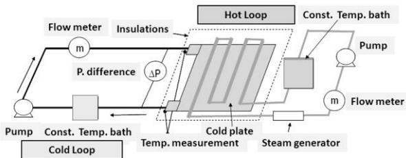
Fig.6 Ground Test Loop of Condenser System
