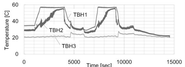
(b) History of temperature in condenser tube (TBH1: Inlet of condenser, TBH2: Outlet of first condensation tube, TBH3: Outlet of condenser )
