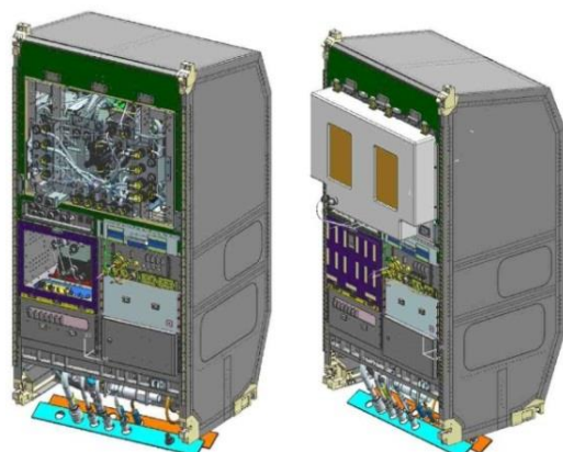
Fig. 3 ELF and UV-Lamp Unit installed in MSPR (Open / Close).
