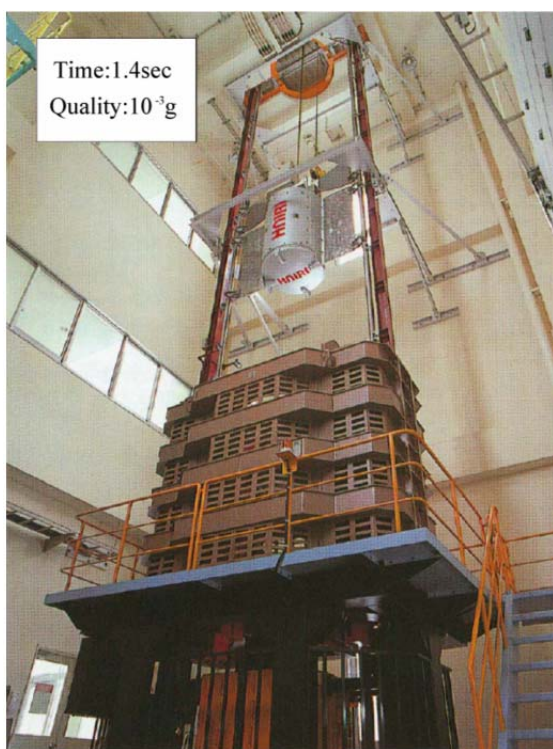
Fig. 1 AIST 10m drop tower.
