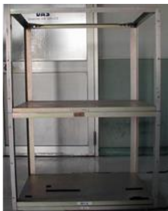
Fig. 4 Experimental rack for 2 instruments (upper and lower space) with the size of 600 \times 500 \times 500 \text{mm}^3
