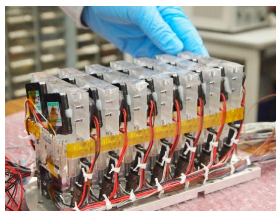
Fig.8 Miniaturized nucleation cells for the detection of nucleation of calcium carbonate crystals. 14 cells were installed, the two of which were used as a test before launch. The scale in figure is in mm.
