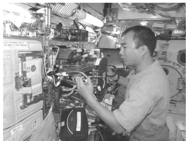
Fig. 7 Setup activity of Marangoni experiment by astronaut Noguchi. (courtesy of NASA)
