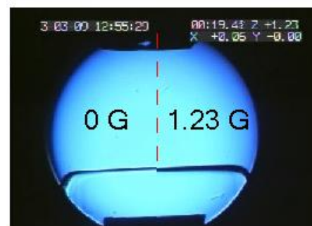
Fig. 12 Crystal shape with c -facet is compared under 0G and 1.23G. The flat surface on the upper side is c -facet. Temperature was 140 mK.
