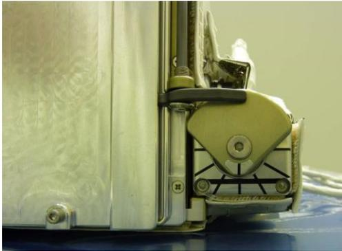
Fig.7 Separation Mechanism on the Case
