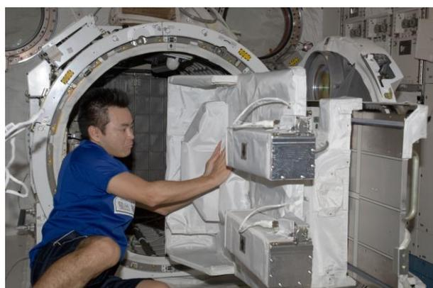
Fig.12 J-SSOD Installation by Astronaut Hoshide
