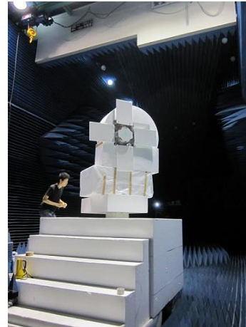
Fig.17 Antenna Pattern Test
