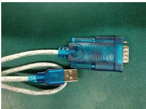
Fig. 6 Serial USB convertor cable
