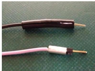
Fig. 10 Connecting sleeves
