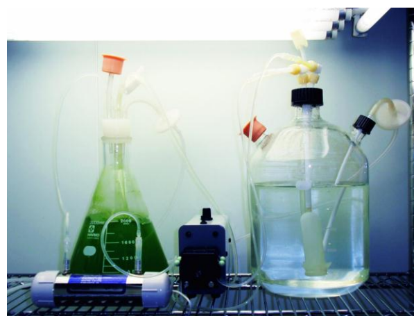
Fig. 5 Nutrient feedback rearing system for water flea. The system is constructed a algal cultivation flask (left side) and a water flea rearing bottle (right side)
