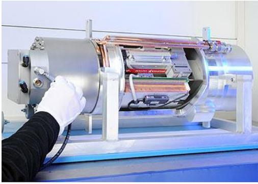
**Fig. 6** Compact and fully MSL compatible X-ray radiography insert for in-situ monitoring of interdiffusion processes under microgravity conditions – on the MAPHEUS sounding rocket and aboard the ISS.
