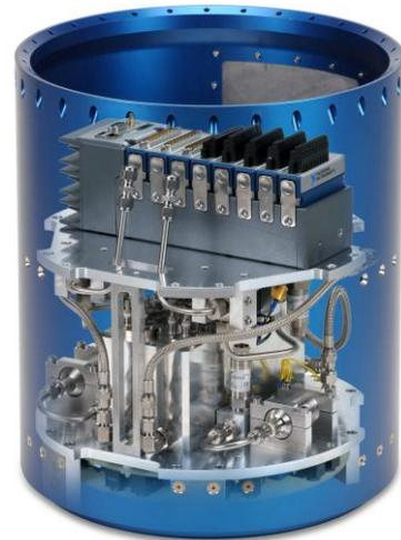
**Fig. 8** MAPHEUS short-time diffusion module ATLAS-M with 8 diffusion furnaces and the MAPHEUS experiment control unit (top). The module's outer radius is 356 mm.
