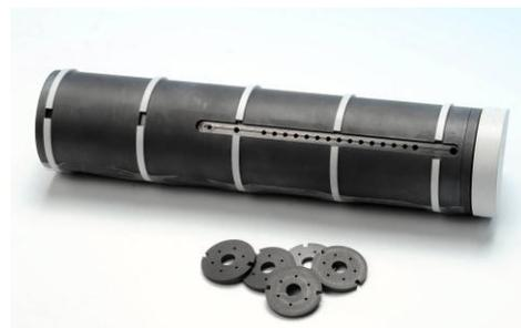
**Fig. 9** Prototype of a 1600°C shear cell comprising of 30, 3 mm thick, shear segments (displayed up front) and bores for up to 6 long-capillary samples.
