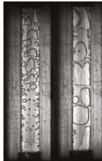
Fig. 7 Flow boiling in a microchannel (upward flow): left: 2g, right: 0g (Image: IUSTI) 17
