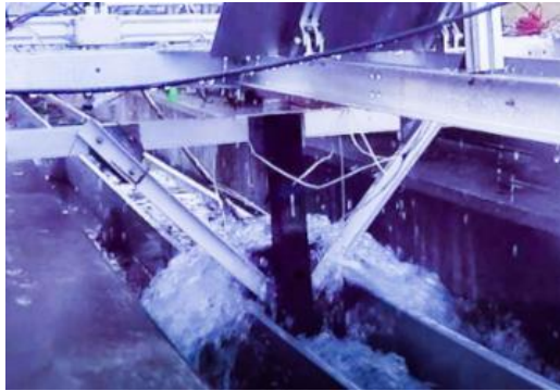
Figure 5. Close up of the water brake in action. (Run 49). 5)
