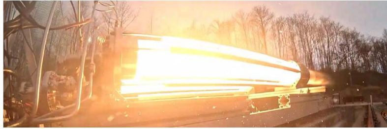
Figure 3. Cluster of two 5-kN class internally developed hybrid motor during launch. (2024)
