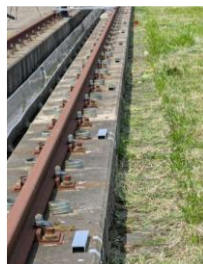
Figure 12. Aluminum channels (30 cm long) were placed beside the rails at 3 meters interval.
