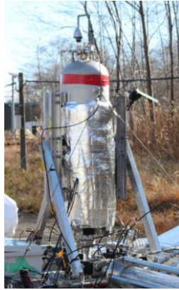
Figure 15. The tank heating system, implemented since Run 68.
