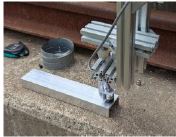
Figure 11. The gap sensor, installed on the sled.
