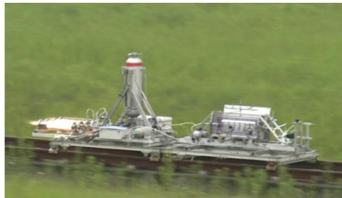
Figure 16. Anti-sloshing tank experiment.
