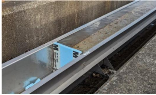
Figure 4. The water channel for water braking, located between the rails. By varying the height of the water gate, the braking force can be controlled.
