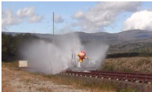
Figure 6. Momentum exchange between the sled and the static water during braking.
