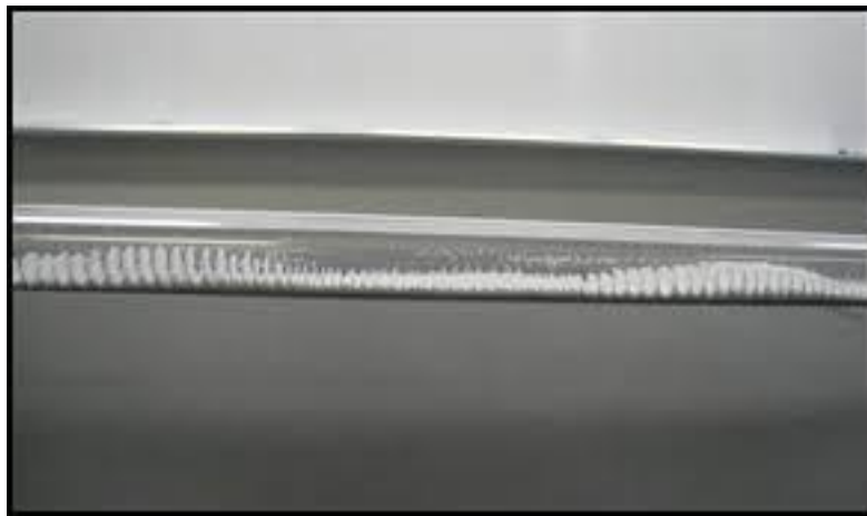
Figure 5. Kundt's experiment under terrestrial gravity conditions 3)
