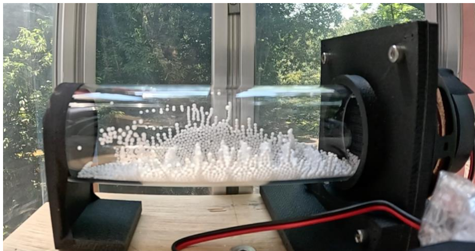
Figure 7. Kundt's experimental equipment immediately before the drop
