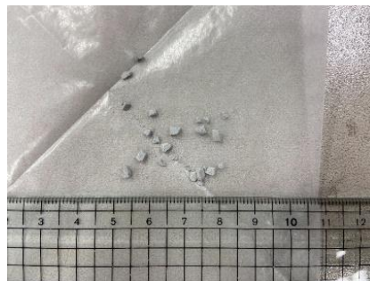
Figure 3. Powdered sample stirred, pressed, and crushed to a size that can float.
