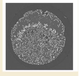
energy of 40 keV. It was shown that internal microstructures were changing depending on the maximum temperature and holding time. When the Al- 10% W alloys were melted at 670 °C for 30 sec, W-based particles were un-uniformly dispersed. Two types of W-based particles, with needle or block-shaped ones, were observed.
