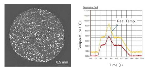
Figure 2. X-ray microtomographic image of Al-10%W (micro-W) after levitation melting at 940°C for 5s.
