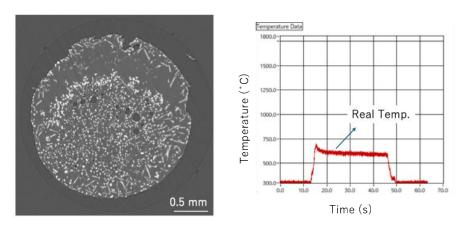
Figure 4. X-ray microtomographic image of Al-10%W (nano-W) after levitation melting at 670 °C for 30s.
