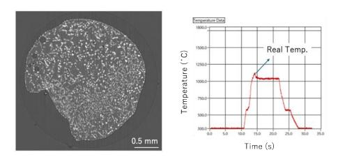
$\textbf{Figure 3}. \ \ \, \text{X-ray microtomographic image of Al-10\%W (nano-W) after levitation melting at 1050°C for 10s.}$
