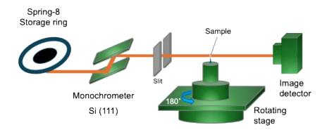
Figure 1. Setup of synchrotron X-ray microtomography in SPring-8 (Beamline: BL20B2).
