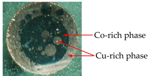
**Figure 2.** cross-sectional structure of Cu-60at%Co taken by optical microscopy
