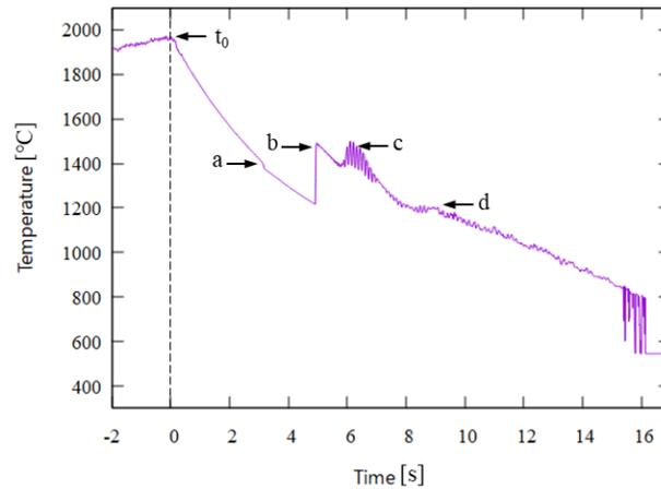
**Figure 1.** temperature data for Cu-60at%Co
