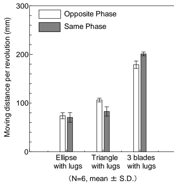
Figure 4. Slip distance per revolution.
