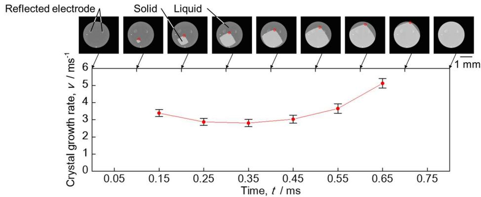
**Figure 1.** Representative series of images obtained by the high-speed camera and crystal growth rate with error. Only the upper vertices indicated by red circles are shown as representatives.
