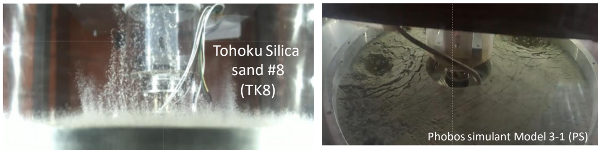
Figure 5. The impact of the pad on each test ground in microgravity (left: TK8, right: PS).
