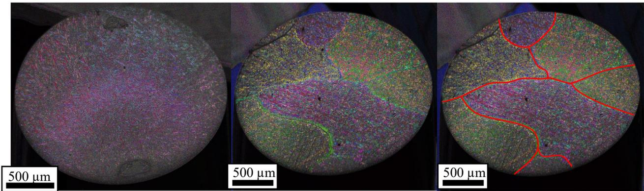
(a)The sample without TiC (b)The sample with 1 vol.% TiC (c)After drawing prior- $\beta$  boundaries on (b)
