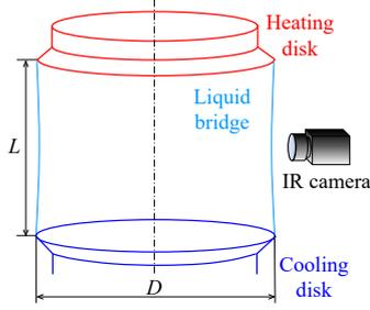
**Fig. 1** Schematic diagram of liquid bridge setup
