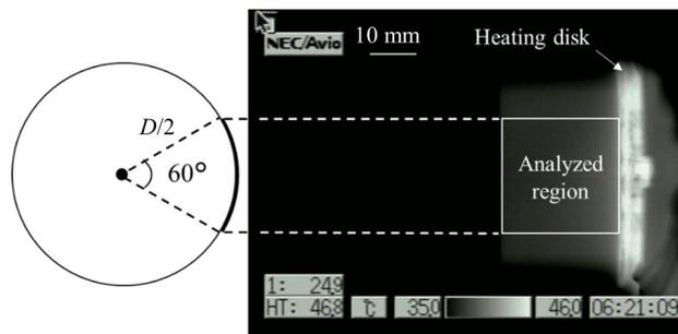
**Fig. 2** Analyzed region of the liquid bridge obtained by the IR camera
