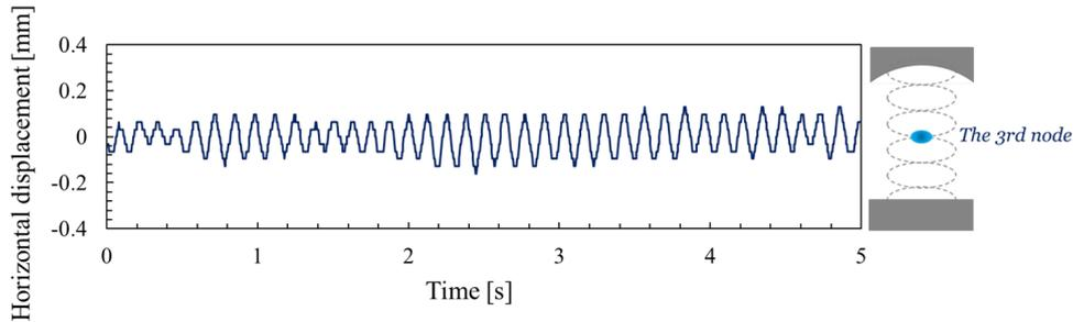
**Figure 2.** Horizontal displacement when a single droplet was levitated at the 3rd node.
