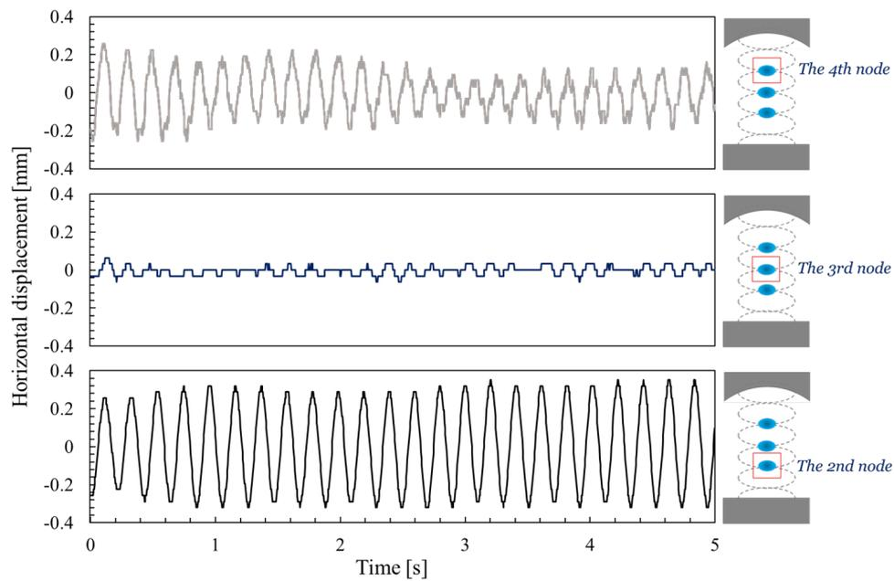
**Figure 4.** Horizontal displacement of three droplets were levitated at the 2nd node, the 3rd node, and the 4th node. The bottom graph shows the results for the 2nd node, the center for the 3rd node, and the top for the 4th node.
