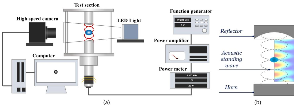
Figure 1. Schematic of acoustic levitator: (a) experimental setup and (b) levitation principle.
