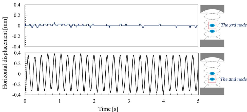
**Figure 3.** Horizontal displacement of the droplet when two droplets were levitated at the 2nd node and the 3rd node. The bottom graph shows the results for the 2nd node and the top for the 3rd node.
