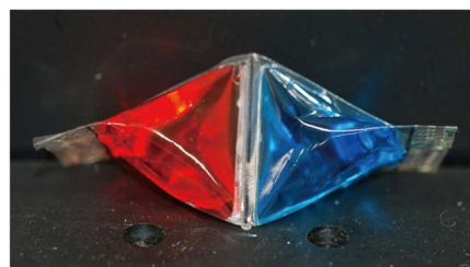
Fig. 4 A sample bag having a breakable separator. Two rooms are filled with red and blue colored liquids.
