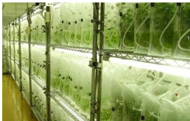
Fig.1 Bag-type culture vessel technology
