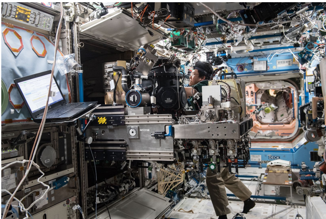
Fig. 1 Japanese astronaut Norishige Kanai reconfiguring a Combustion Integrated Rack (CIR) camera [ISS055e096568]
