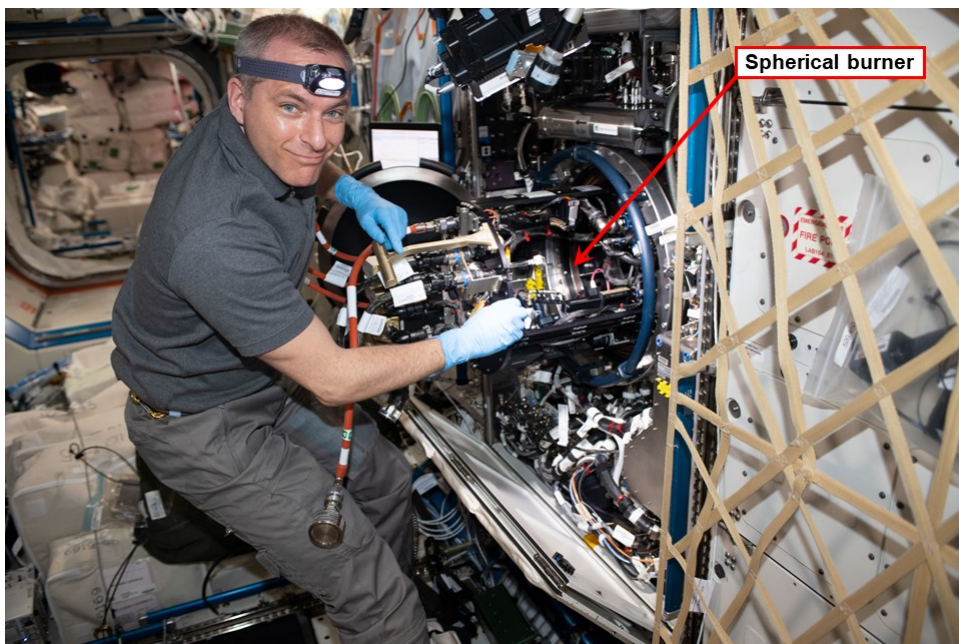
Fig. 3 Canadian astronaut David Saint-Jacques working with the ACME chamber insert [ISS059e060847]
