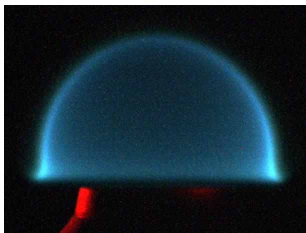
Fig. 7 Pure ethylene BRE flame, where the burner is illuminated from the left in red
