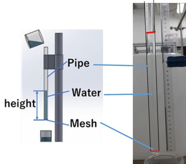
Fig.2 Test piece for bubble point test
