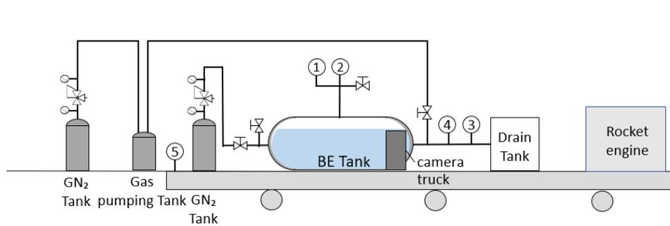
Fig.8 The piping diagram of the experiment.
