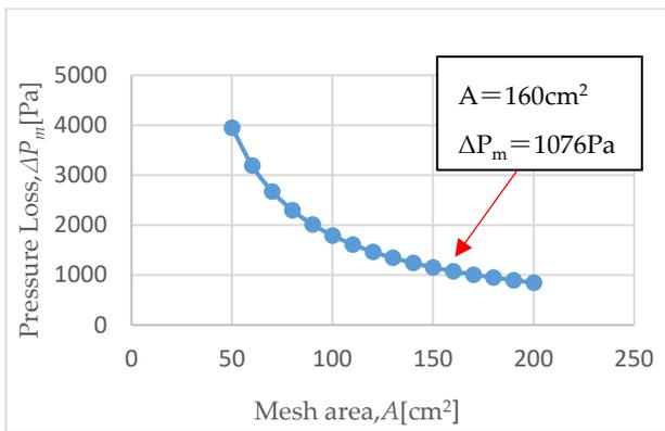
Fig.3 Changes in mesh surface area and pressure loss
