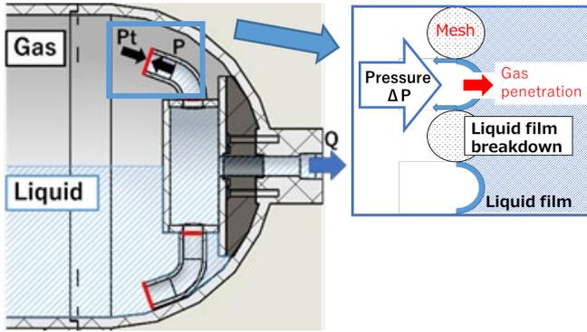
Fig.1 Installation of propellant management device
